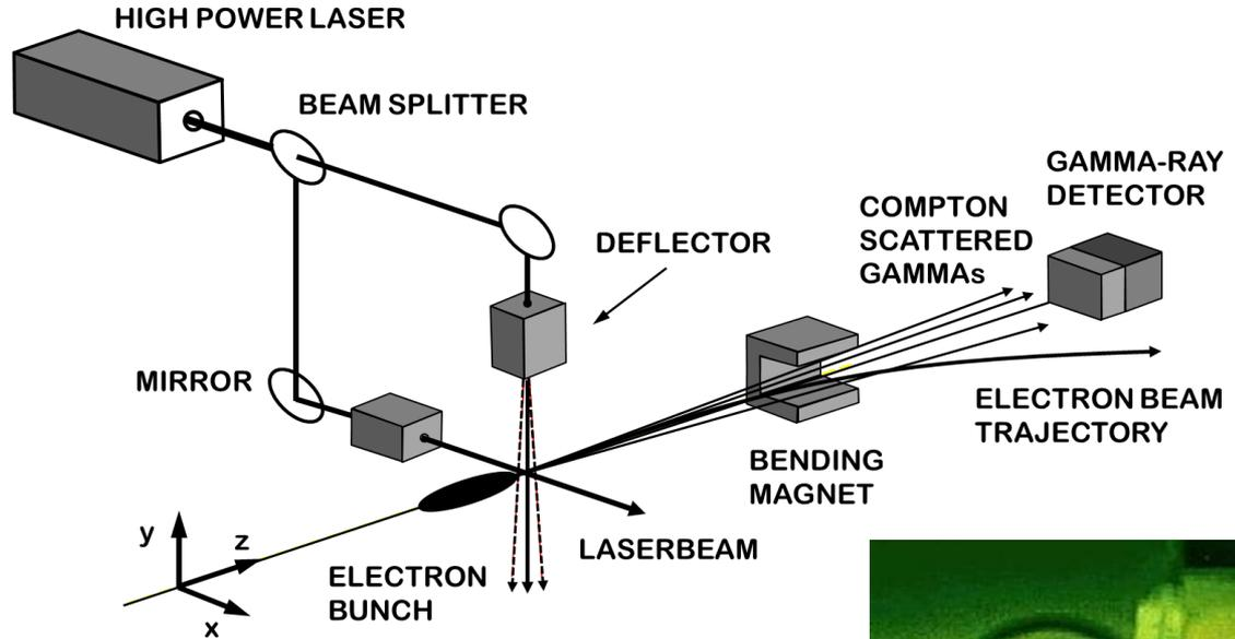
Beam profile monitor with laser beam as the "wire"
