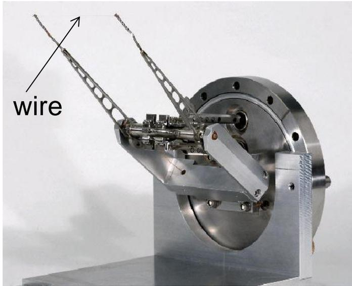
Beam profile monitor with tungsten or carbon wire
