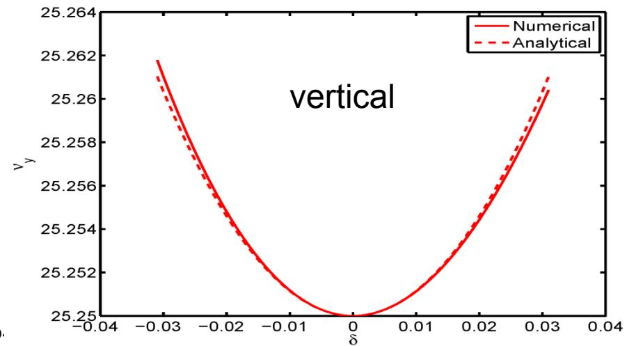
Comparison to a numerical simulation in LEGO in a ring that consists of 101 90° cells.
