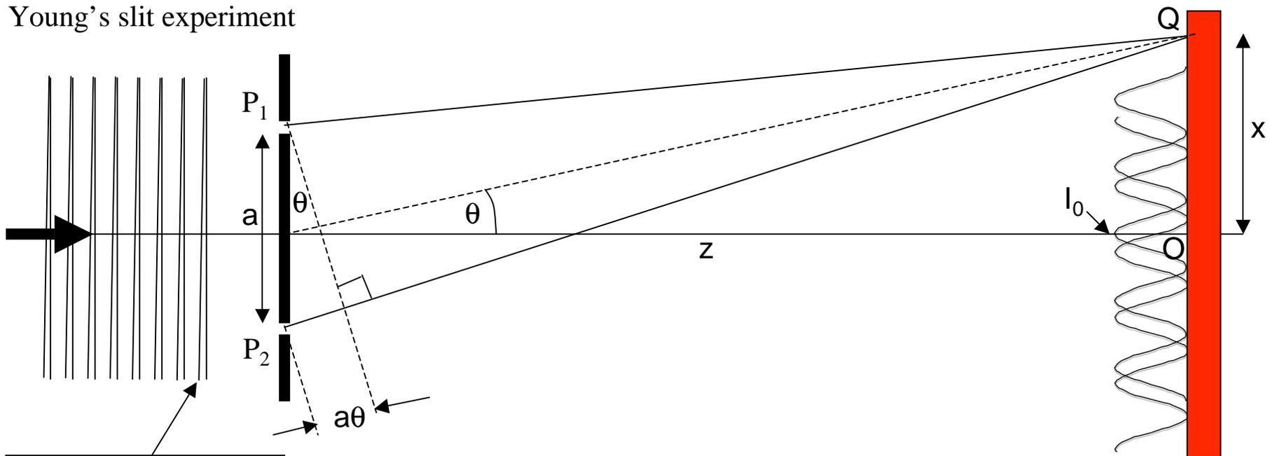
Second wave tilted by  $\varepsilon = \lambda/(4a)$  giving an additional path lag of  $\lambda/4$  of the signal from  $P_2$  relative to that from  $P_1$
