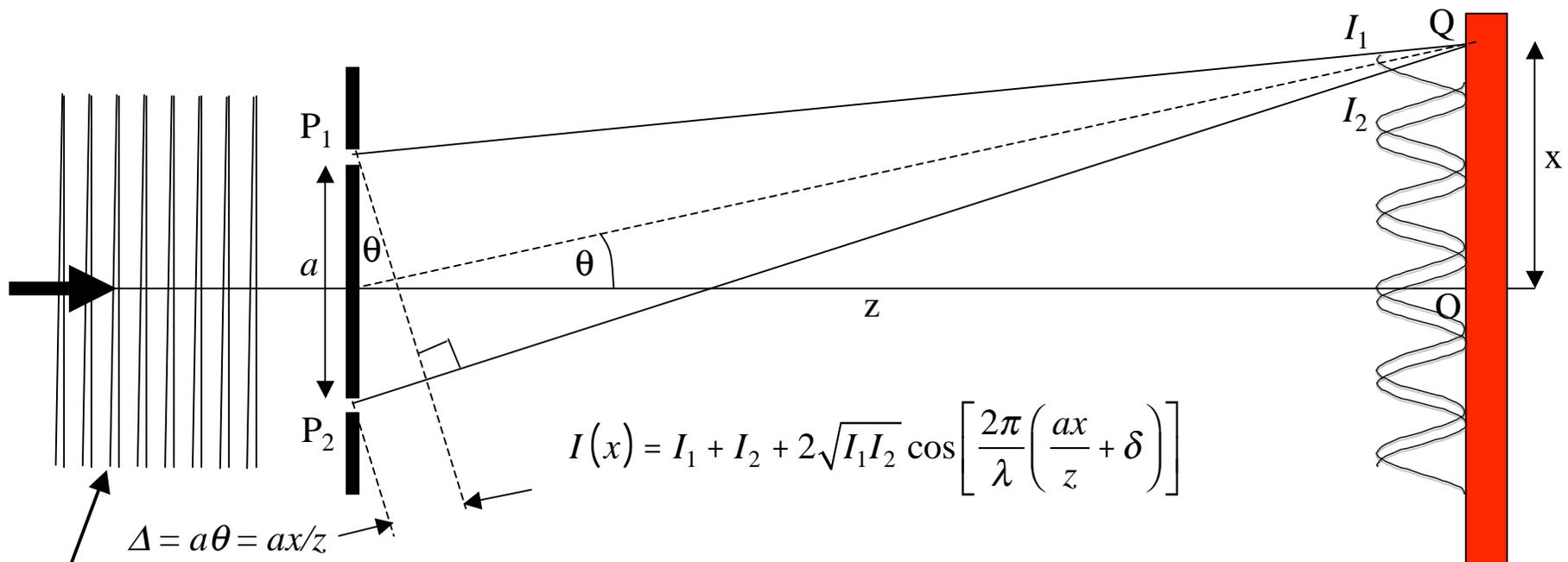
$$I(x) = I_1 + I_2 + 2\sqrt{I_1 I_2} \cos \left[ \frac{2\pi}{\lambda} \left( \frac{ax}{z} + \delta \right) \right]$$
