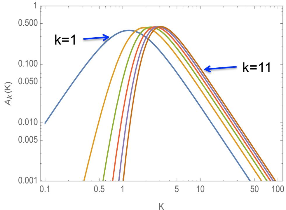
Undulator parameter K should be between 1 to 4
