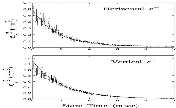
Figure 2. Sample of data for the positron damping ring. The vertical scale represents the real size of the bunch.
