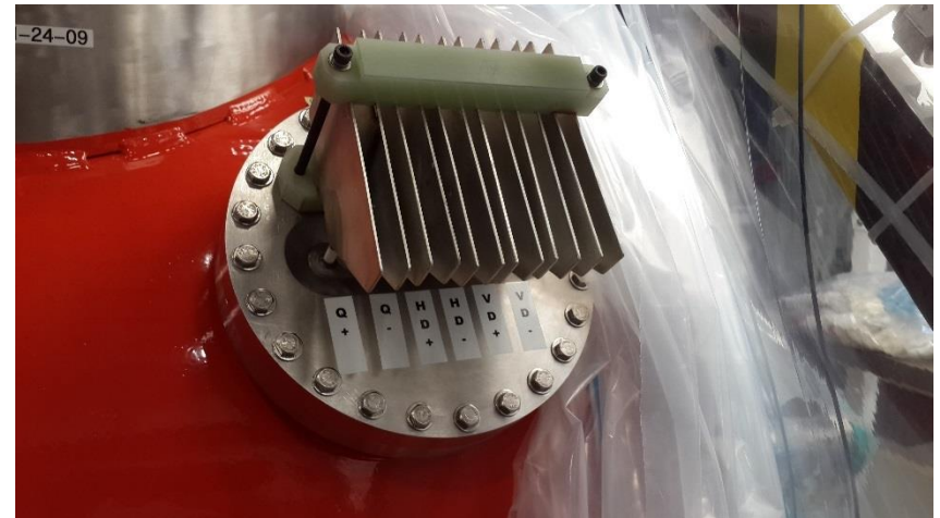
External power leads flags.
