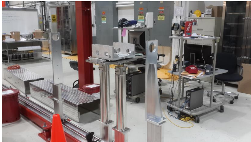
Post for clamping magnet around a beam pipe in MP9.
