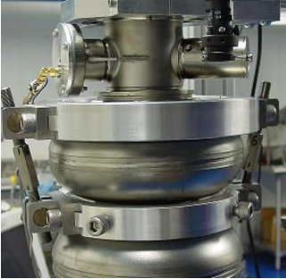
“Iris”, axial tuning fixture
