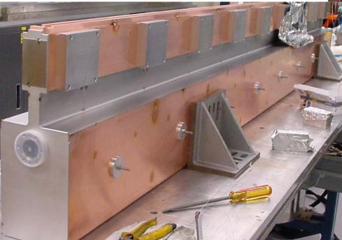
C10100 <sup>1</sup>/<sub>2</sub>-Hard Cu sheet bend to U-box to form a TiSP pumping plenum
