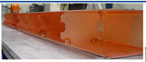
C10100  $\frac{1}{2}$ -Hard Cu plates machined to form a beam pipe
