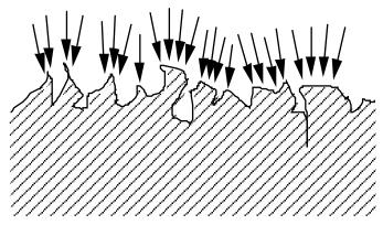
Resulting surface has reduced peaks, reduced surface area, and reduced outgassing
