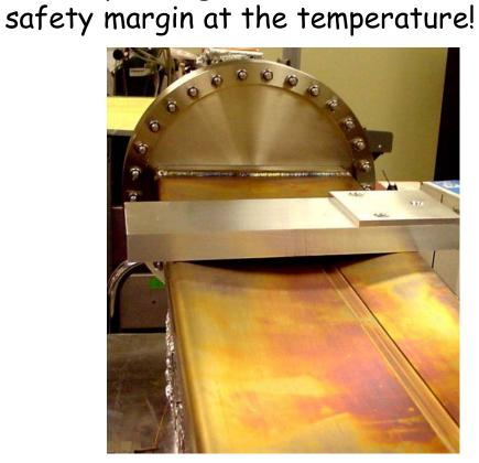
Distorted copper chamber during a bakeout
