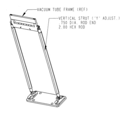
This stand provides support and adjustment capability in the y-direction and roll.
