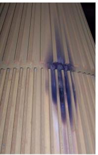
Electron beam melted through aluminum body
