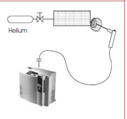
d: Local leak detection; pressurized test gas inside the specimen
