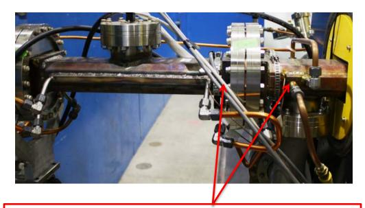
TCs between cooling, most common locations. Many clogged lines, dead-looped plumbing were "discovered" by the TCs.
