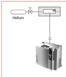
a: Integral leak detection; vacuum inside specimen
