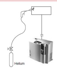
b: Local leak detection; vacuum inside specimen
