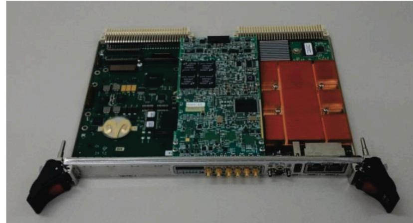
Figure 2: Digital LLRF PMC board and VME board.
