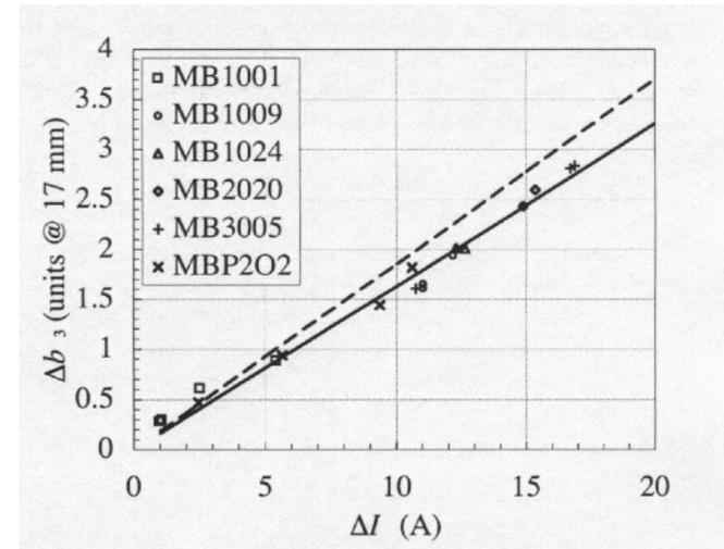
Linear relation between snapback constants for Tevatron (right) and LHC (left) dipoles from L. Bottura et al, IEEE Trans. Appl. Supercond. **15** (2005) 1217-20.
