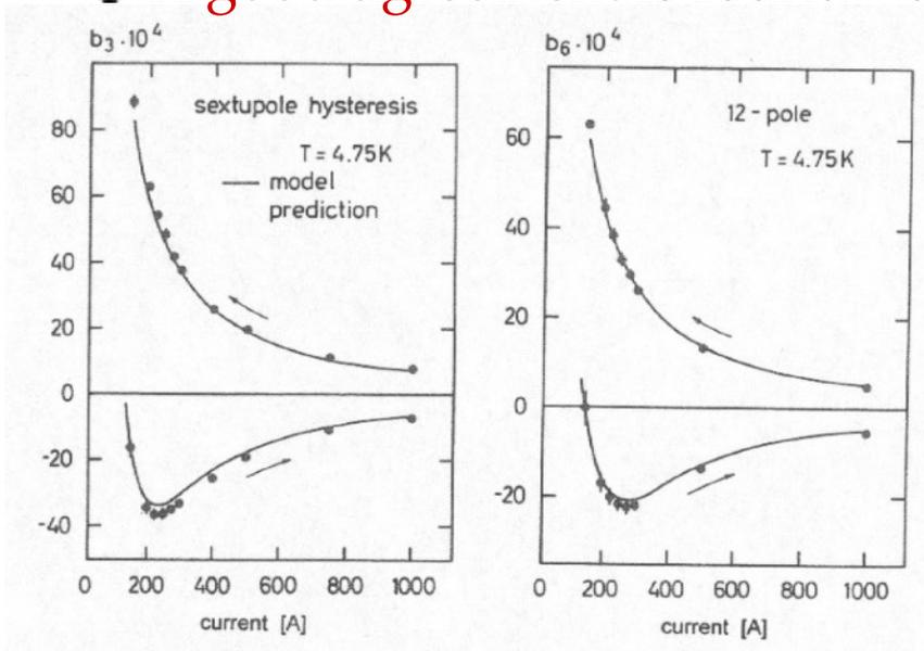
Persistent current measured vs computed in HERA dipoles and quadrupoles - From P. Schmuser, pg. 87 Fig. 6.5
