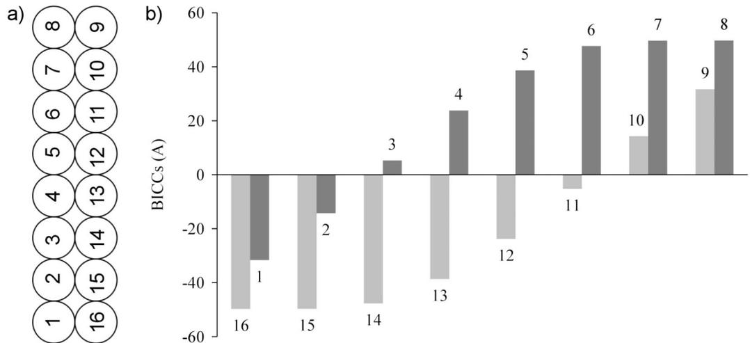
Figure 2.19 a) Numbering of the strand positions in the cross section of a 16-strand Rutherford-type cable. b) Illustration of the BICC magnitude in a 16-strand cable at a certain  $z$ -position. The labels indicate the strand positions [55].
