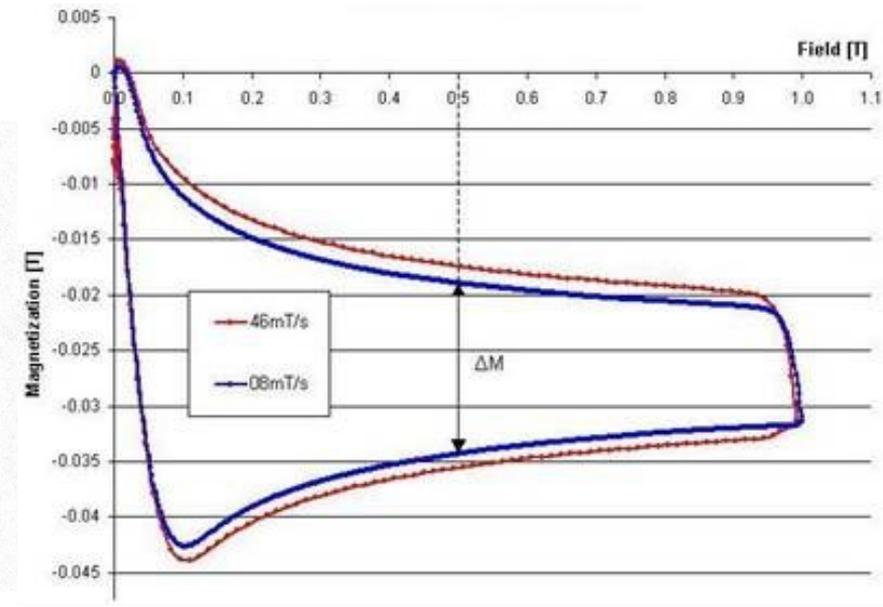
Magnetization measurement in LHC cable
