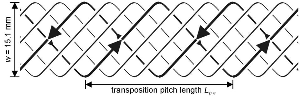
Figure 2.18 Two strands in a Rutherford-type cable carry a current, flowing in a long loop.
