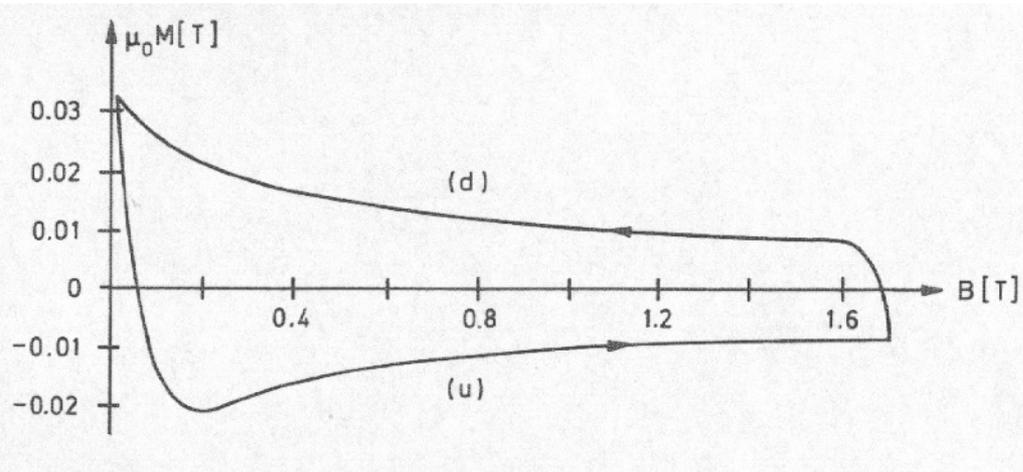
Magnetization measurement in HERA cable
