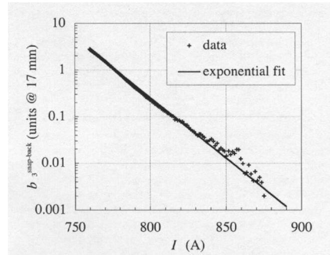
Snapback in  $b_3$  versus time, LHC main dipoles, from L. Bottura et al, IEEE Trans. Appl. Supercond. **15** (2005) 1217-20.
