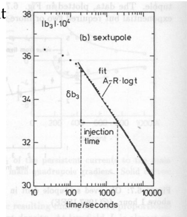
Decay of  $b_3$  in HERA dipoles versus time, from Schmuser pg. 90, fig 6.8
