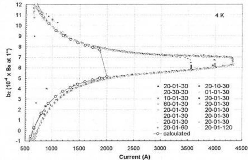
Persistent current measured vs computed in Tevatron dipoles - From P. Bauer et al, FNAL TD-02-040 (2004)
