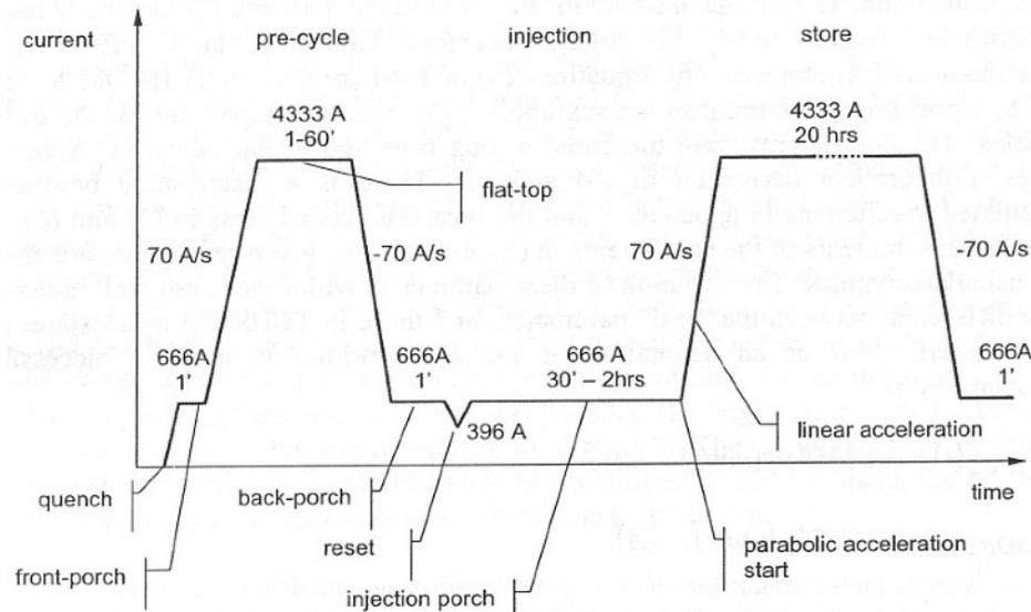
The cycle used for powering Tevatron dipoles, from P. Bauer et al, FNAL TD-02-040 (2004)
