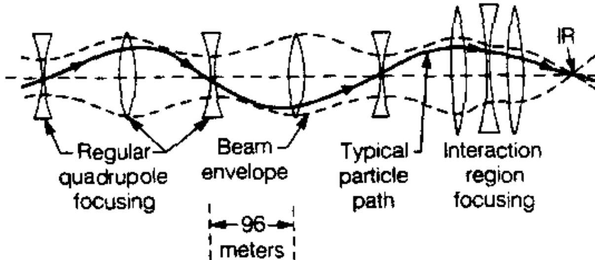
A standard cell is typically a quadrupole followed by several dipoles, then a quadrupole of the opposite focusing characteristic from the first and another set of bending magnets equal in length to the first. Referred to as a FODO cell.
