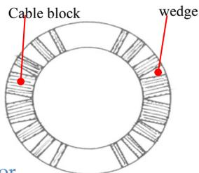
A practical winding with one layer and wedges
