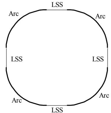
A schematic view of a synchrotron
