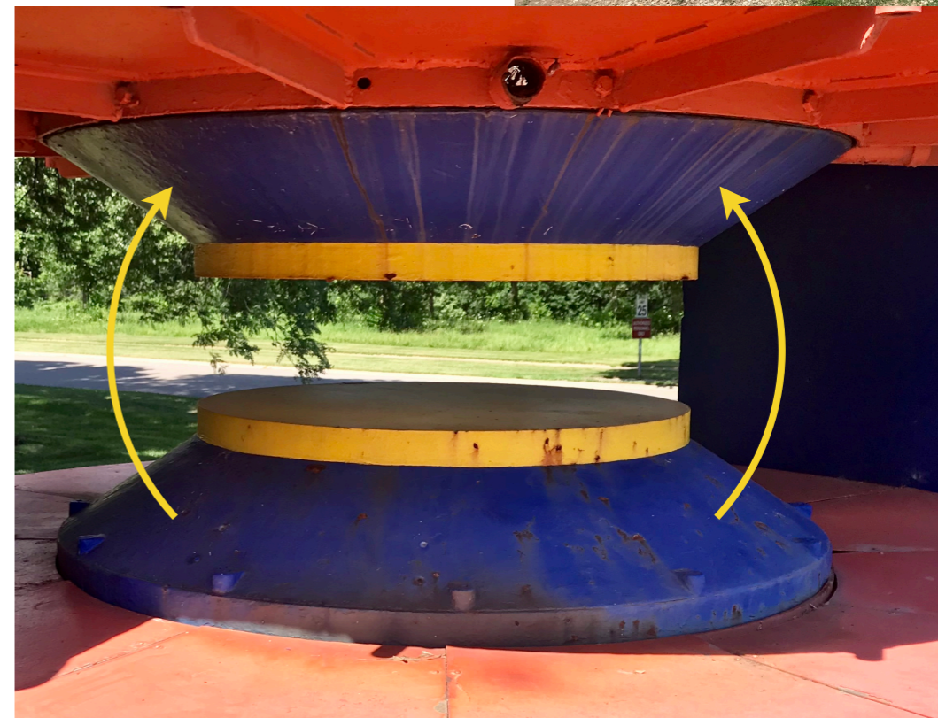
1935 U. Chicago cyclotron magnet, Fermilab Village
