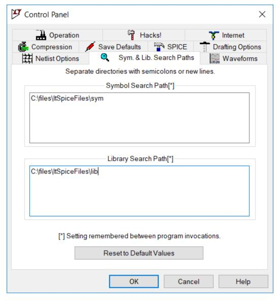
We will be creating IGBT files, so copy the standard symbol for an N channel IGBT into the C:\files\ltSpiceFiles\sym directory. From C:\LTC\LTspiceXVII\lib\sym\Misc copy NIGBT.asy and PIGBT.asy to
