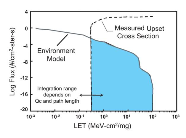
Measured upset error cross section and particle flux for a hypothetical space environment. The error rate is determined by convolving the environment model with the error cross section. [J. R. Schwank, M. R. Shaneyfelt and P. E. Dodd, "Radiation Hardness Assurance Testing of Microelectronic Devices and Integrated Circuits: Radiation Environments, Physical Mechanisms, and Foundations for Hardness Assurance," in IEEE Transactions on Nuclear Science, vol. 60, no. 3, pp. 2074-2100, June 2013.]
