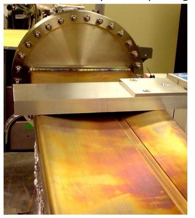
Disformed copper chamber during a bakeout The chamber was saved by pressurizing and stiffening
