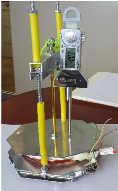
HTS Coil test setup
