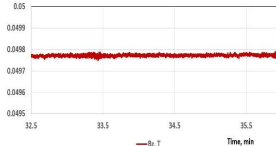
HTS Coil field stability was ~0.5 Gauss
