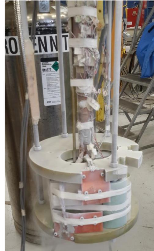
HTS Quadrupole Test Setup
