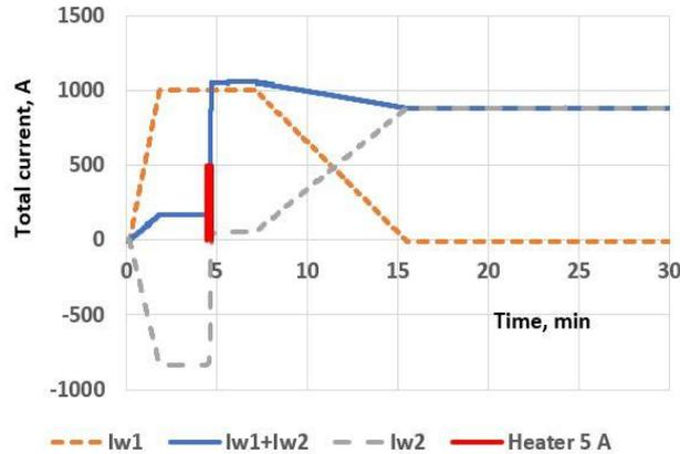
In secondary HTS Coil induced -833 A current
