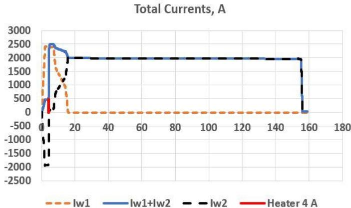
In secondary HTS Coil induced -1900 A stable current
