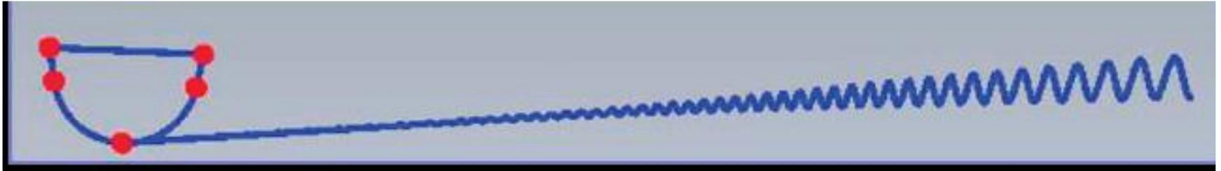
Sweeping vane tip profile along modulation curve.
