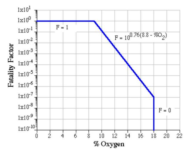
**Figure 1** Fatality factor F<sub>i</sub> versus the lowest attainable oxygen concentration that can result from a given event (derived from *Fermilab Environment, Safety, and Health Manual*, Chapter 4240, "Oxygen Deficiency Hazards [ODH]" [FESHM 4240])
