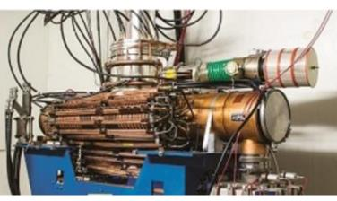
Tunable cavity for FNAL Booster Synchrotron
