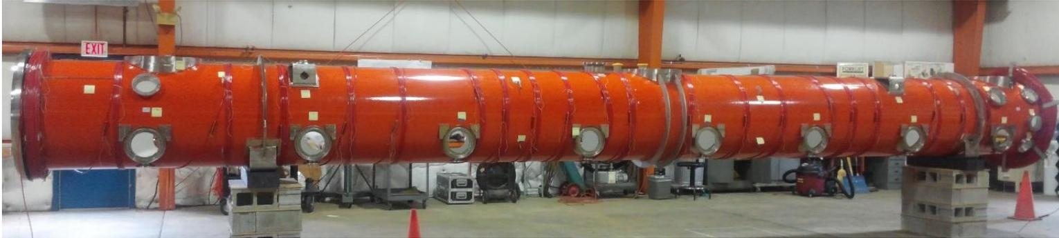
Helmholtz coils wound onto vessel directly
