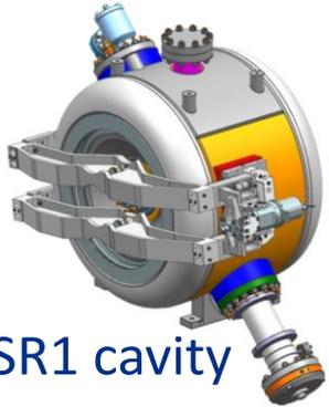
Strong MP in SSR1 at 5, 6.5 and 7 MV/m. 120 C bake for 48 h helps to reduce MP conditioning time
