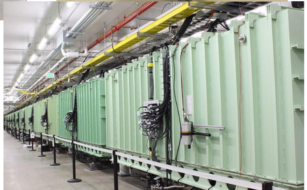
5-cell 644 MHz cavities for FRIB upgrade
