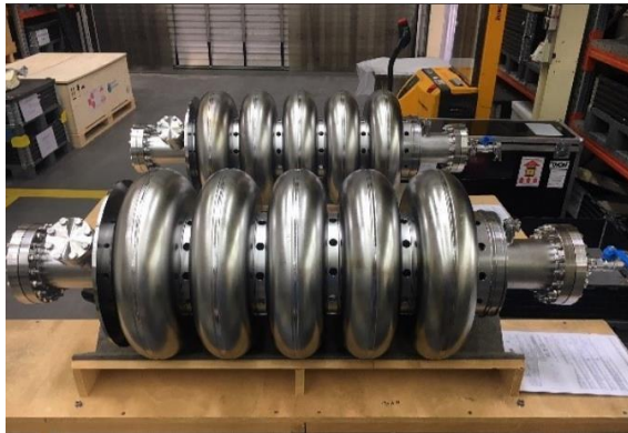
5-cell 644 MHz cavities for FRIB upgrade
