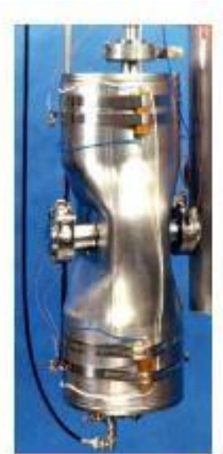
The first 355 MHz SC HWR ANL - \beta=0.12
