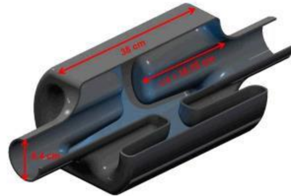
Superconducting 4-rod cavity
