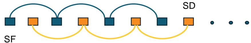
Wiring of sextuples for chromatic beta beat correction (W function) for a 90 deg lattice:
