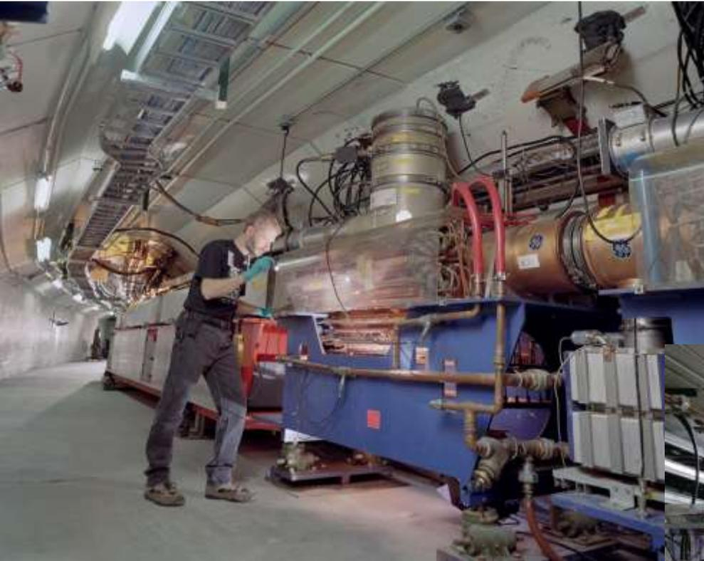
Two 8 GeV pbar rings for stochastic cooling in one  $\Delta$ -shape tunnel
