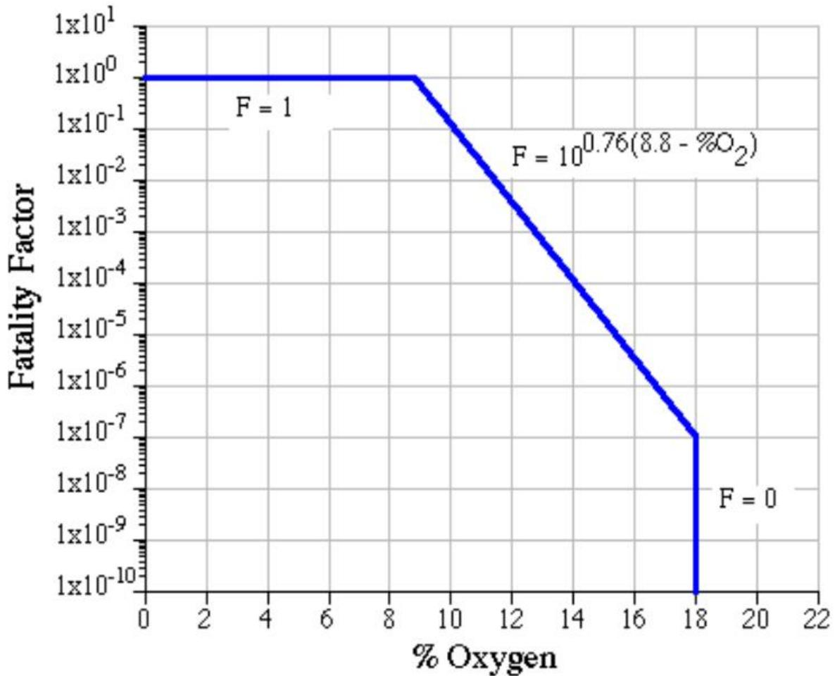
Figure 1 Fatality factor  $F_i$  versus the lowest attainable oxygen concentration that can result from a given event (derived from *Fermilab Environment, Safety, and Health Manual*, Chapter 4240, "Oxygen Deficiency Hazards [ODH]" [\[FESHM 4240\]](#))
