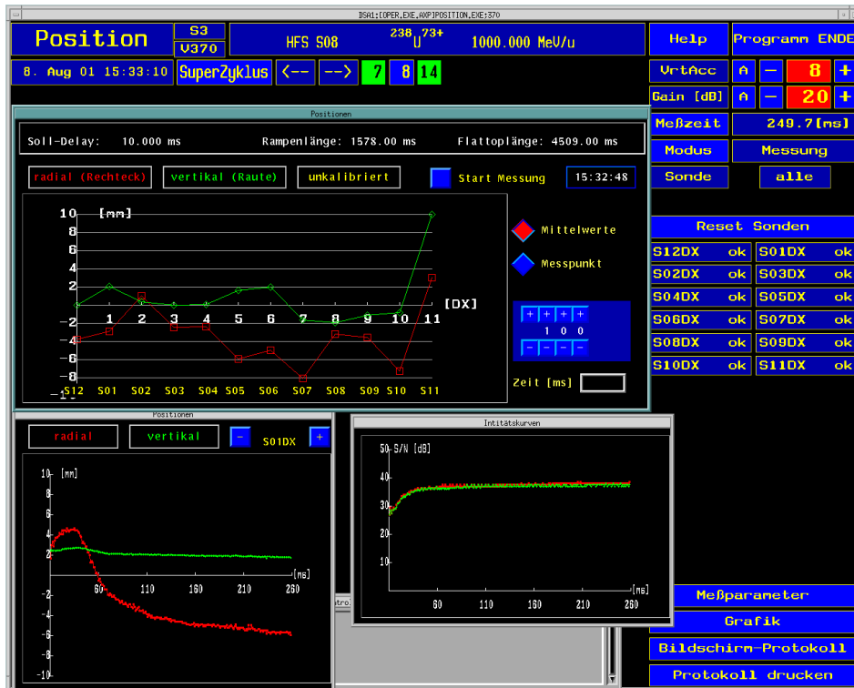
Figure 5.27: Example of a position measurement done at the GSI synchrotron for a partly misaligned beam during the acceleration. The top plot shows the position around the ring at a certain time, the lower left is the position for one pick-up and the lower right is the sum signal power \propto U_{\Sigma}^2 during the ramp for the same single pick-up.
