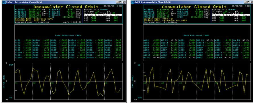
Figure 1.8. Difference orbits showing oscillations about the machine design orbit caused by dipole deflections. The plot on the left shows a horizontal deflection. The plot on the right shows a vertical deflection.
